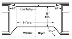
Side-by-Side Units in Under-Counter Installation Requires custom-built countertop and/or cabinetry.
